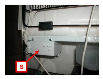
Starting from the contact 9 of the connector J1 (connected to the power board) follow the path of the cable (in the fig. of blue colour) up to the connector for the connection of the thermal switches K (featured in the connection box of the compressor compartment S). 2. Access to the connection box S.
