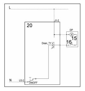
The PCB powers the drain pump via a triac as follows:
