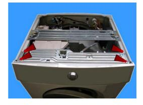
Unscrew the screws which fit the control panel to the detergent dispenser.
