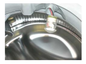
While reassembling, pay attention that the clamp that fixes the lamp to the rubber bellow is positioned correctly, the exceeding part is perfectly cut (as indicated by the arrow in Fig. A) and the wiring is placed (as in fig. B).
