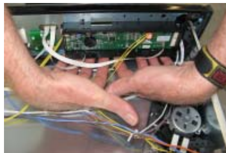
Unlatching the detents by gripping underneath with both hands.
