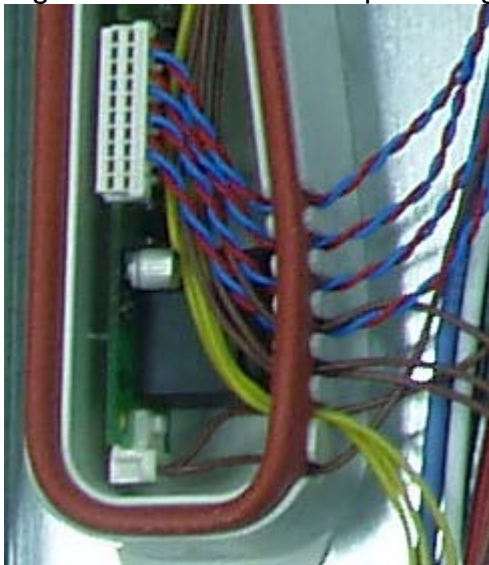
Fig. 22: Wiring with pot recognition electronics
