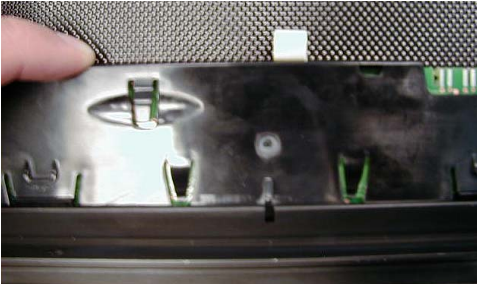
Fig. 13: ... and press it against the front of the frame so that the projection fits into the recess. It must audibly lock into place.
