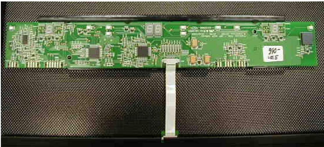
Fig. 10 Stripline plugged in and latched in position at the electronics and the keyboard
