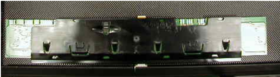
Fig. 11: Fold the electronics up with the display on the glass side
