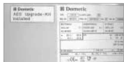
Attach sticker "AES Upgrade-Kit installed" next to data plate.
