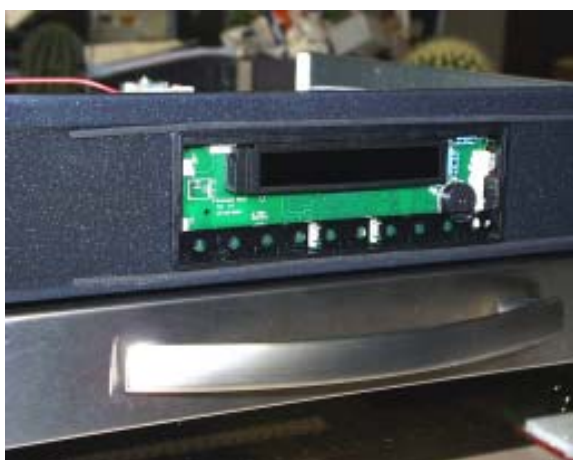
Fig.: Input electronic in installed condition and disassembling after unlocking
