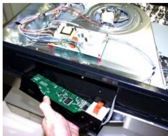
Fig.: Input electronic in installed condition and disassembling after unlocking
