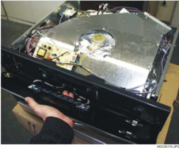
Fig. 44 : Switch panel after disassembly
