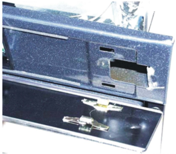
Fig. 45 : Support springs switch panel
