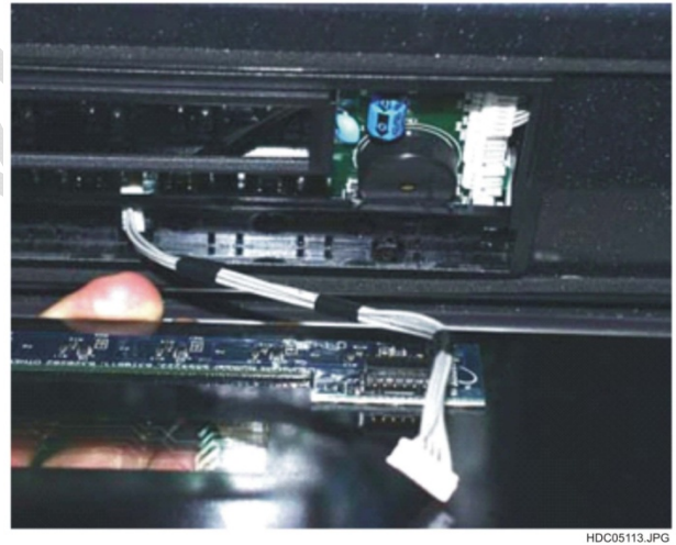
Fig. 47 : Removed data link
