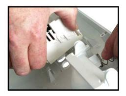
The electronics can then be snapped out.
