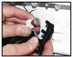
The mounting for the thermostats is screwed in behind the leach pump.
