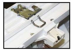
After removing the spring, the door-opener can be removed from its hinges.
