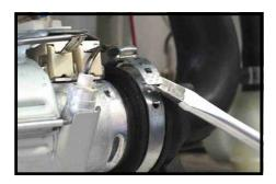
To release the hose clamps, it is recommended that this assembly be taken off its hinges.
