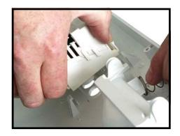
The electronics can then be snapped out.
