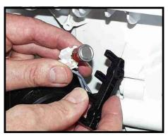
The mounting for the thermostats is screwed in behind the leach pump.
