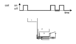
During the rinse cycle, the coil is always switched on twice. When it is switched on the second time, the remaining rinse-aid flows into the rinse tank.
