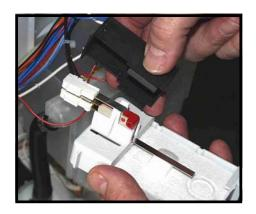
The flooding switch is snapped out with a small screwdriver and can be taken out of its mounting.
