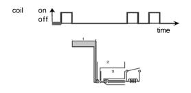
During the washing cycle the coil is switched on and the detergent compartment cover releases the detergent. The rinse-aid flows from compartment 1 into compartment 2.
