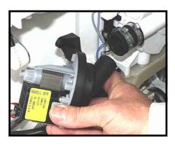
To dismount the leach pump, the hose clamps are released and the screws removed.
