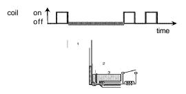
During the rinse cycle, the coil will be switched on when the rinse is warmed and the rinse-aid runs from compartment 3 into the rinse tank. At the same time, the remaining rinse-aid (15%) runs from compartment 1 into compartment 2.
