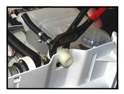
After the removal of the hose, the valve can be drawn out of the chassis with suitable pliers.
