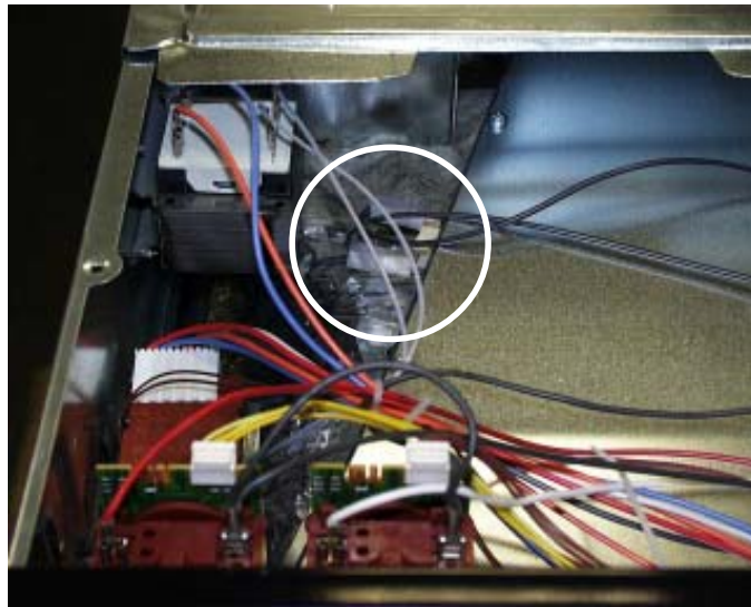
Fig.: Built-in position - Temperature fuse
