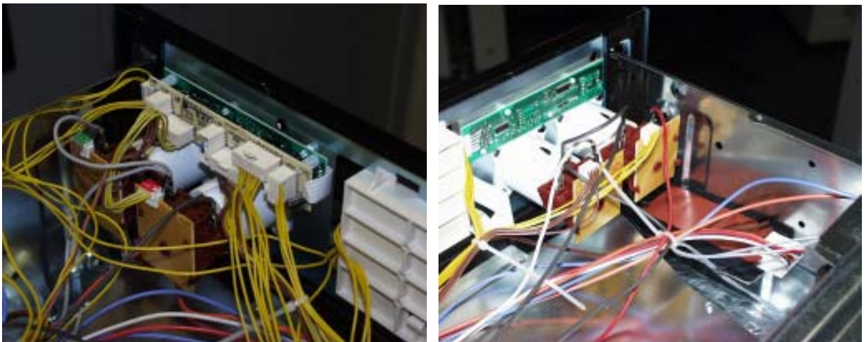
Fig.: input electronic HOC2000 and Input module in installed condition
