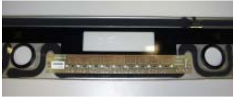
Fig. Touch board stuck with switch panel
