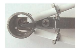
Due to production tolerances it might happen that the space between the ignition plug and the bottom of the burner housing is too small. Thus, a correct ignition is not always possible, as the spark might jump over to the burner housing.
