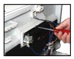
The door lock and the dosing unit is held by screws.
