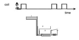
During the washing cycle the coil is switched on and the detergent compartment cover releases the detergent. The rinse-aid flows from compartment 1 into compartment 2.
