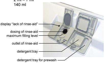
The detergent compartment 1 is filling corresponding to the set dosing quantity when the door is open. Possibly existing rinse-aid in compartments 2 and 3 flows back into the storage tank of the rinse-aid. The detergent trays are filled up. The door will be closed and the detergent for prewash will be rinsed out through the slots in the detergent dispenser cover.
