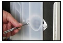
To dismount the water softener, these attachment screws are removed.
