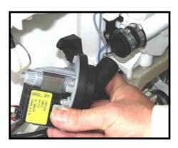
To dismount the leach pump, the hose clamps are released and the screws removed.
