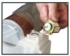
After undoing the screws of the recycling valve, this can be removed.
