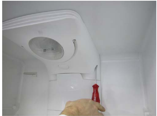
b) 2 screws in the rear part
