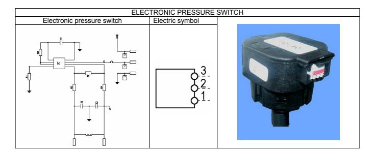
The pressure switch is connected by a hose to the pressure chamber.
