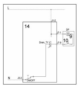
The PCB powers the drain pump via a triac as follows:
