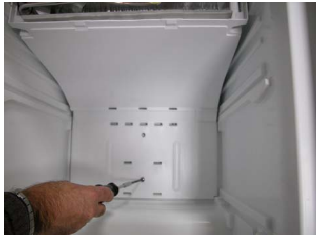
i) Unscrew the 2 fixing screws of the air diffuser.
