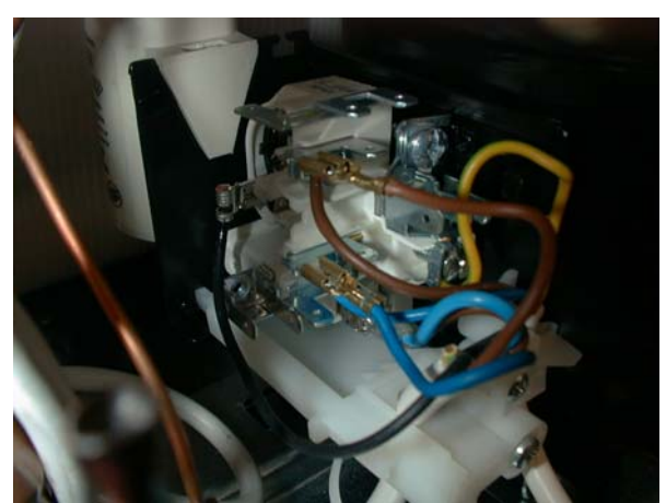
d) View of the internal components: • compressor terminal box
