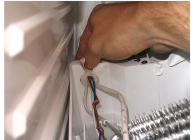
s) Remove the sealing rubber.
