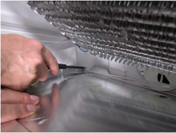
p) Release the left hook of the defrosting heater.
