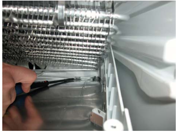
q) Release the right hook of the defrosting heater.
