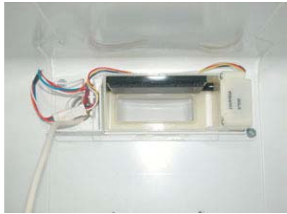
f) The damper is fitted with 2 screws and is connected to the electric wiring by means of a 4-pole connector
