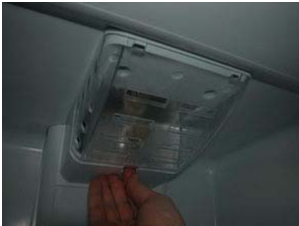
a) Remove the lamp protection by releasing the hook
