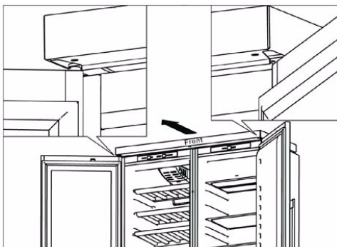
c) Remove the steel plate cover from the hinges as indicated by the arrow
