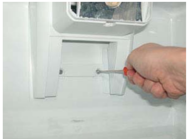
d) Unscrew the 2 front fixing screws
