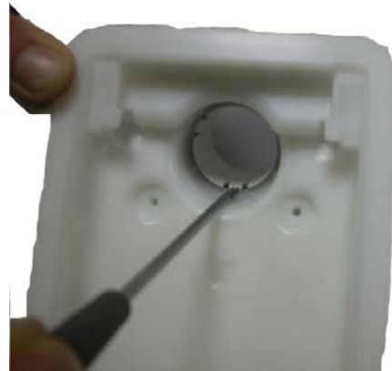
f) remove the internal protection housing by means of a screwdriver
