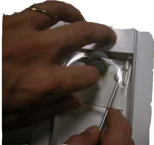
b) release the water distributor lever by means of a screwdriver
