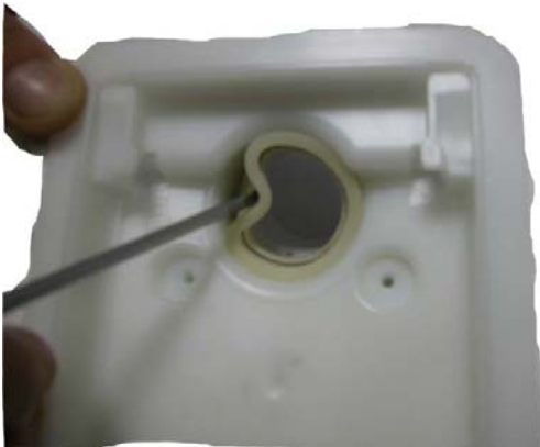
e) remove the valve basket by means of a screwdriver
