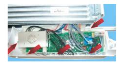
c. Before mounting the new board extract the knob pressing the hooks indicated by the arrows as represented in figure.
