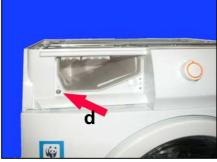
e. Cut the clamp which secures the wiring to the board casing (while reassembling, put a new clamp).
