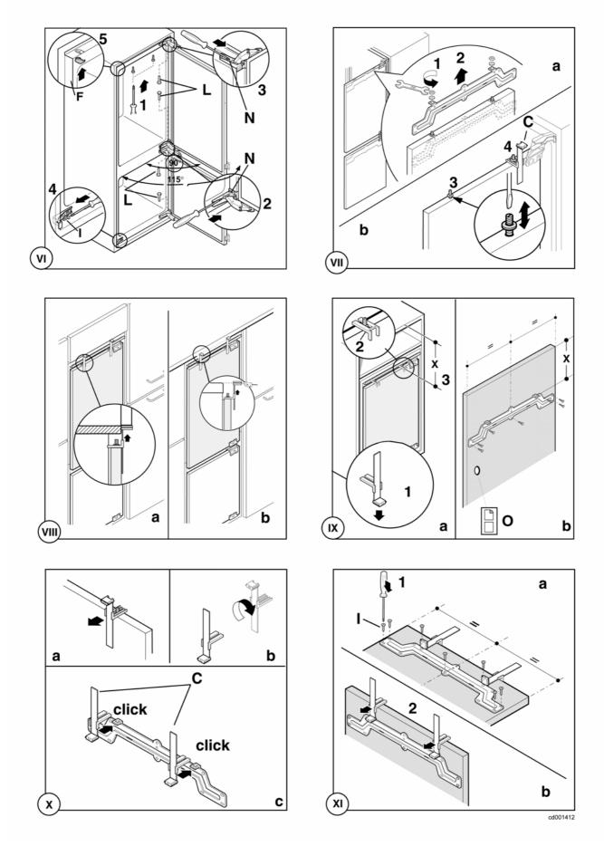
COMPONENTS FOR THE INSTALLATION OF BUILT-IN MODELS WITH "DOOR ON DOOR" SYSTEM 9/10
