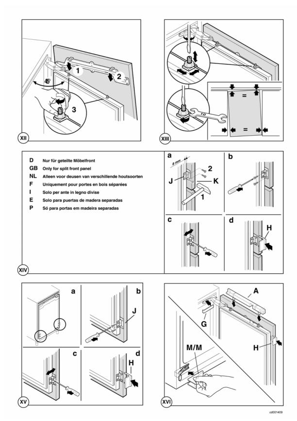
COMPONENTS FOR THE INSTALLATION OF BUILT-IN MODELS WITH "DOOR ON DOOR" SYSTEM 6/10
