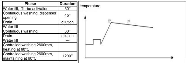
**N.B.**: At the beginning of the subsequent programme (i.e. after the test cycle), the resins are washed. The overall duration of the test cycle is about 15 minutes.
