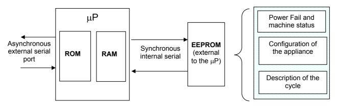
The main circuit board features an EEPROM memory (external to the microprocessor) which stores in memory data relative to the configuration, description of the cycle, cycle status in case of a power failure, and any alarm conditions.
