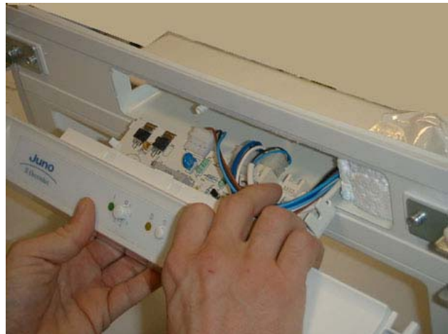
b) Remove the wiring as indicated in picture;
