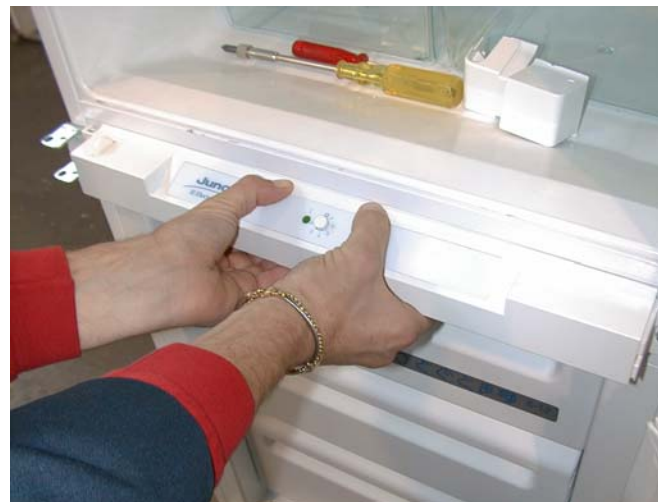
h) Remove the control panel from the intermediate crossbar;
