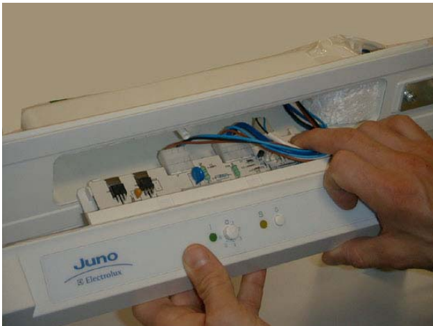
c) Put the control panel close to the intermediate crossbar and keep the wiring aside;
