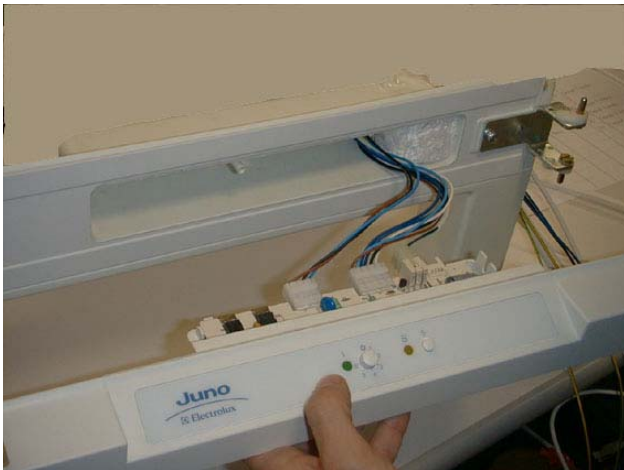
a) While remounting the control panel be careful with the wiring because it could interfere with the board connectors;
