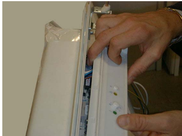
d) Put the control panel close to the intermediate crossbar and keep the wiring aside;
