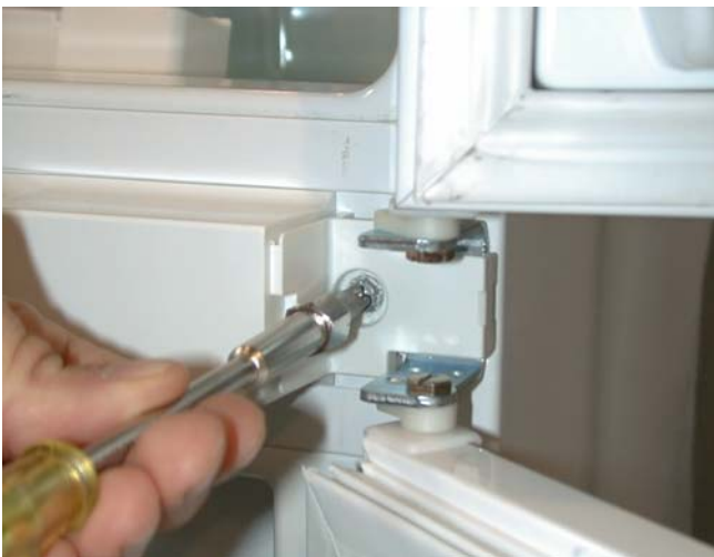
g) Remove the fixing screws of the control panel;
