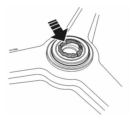
Fill entirely with grease the inside of the seal!
