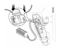
Fit the thermostat casing in position and then the heating element to the compartment using the screw included in the kit.
