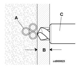
Use an 8mm bit to drill the hole paying attention not to overcome the compartment shim in order to avoid any damage of the foamed wiring behind the compartment!
