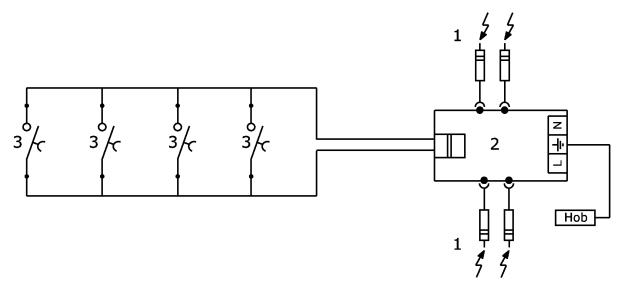
1 Spark plug for ignition2 Ignition With Terminal Box3 Switch for ignition
